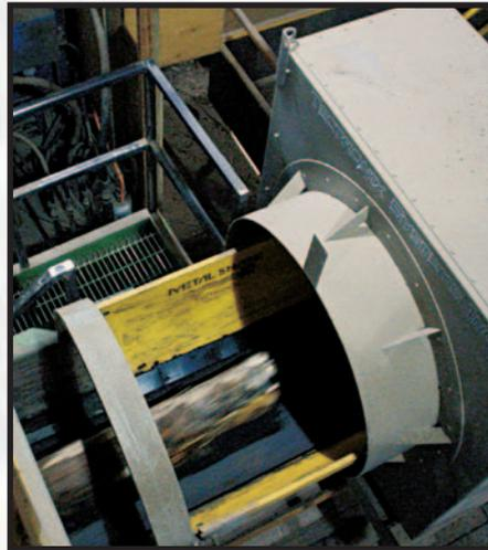
signal has to be extracted from a much larger signal and within that larger signal is the product signature as well as any mechanical or electrical noise signals. DSP allows for filtering or differentiation of the different signatures or signals so that metal can be recognized for what it is without degradation to the performance of the system.
